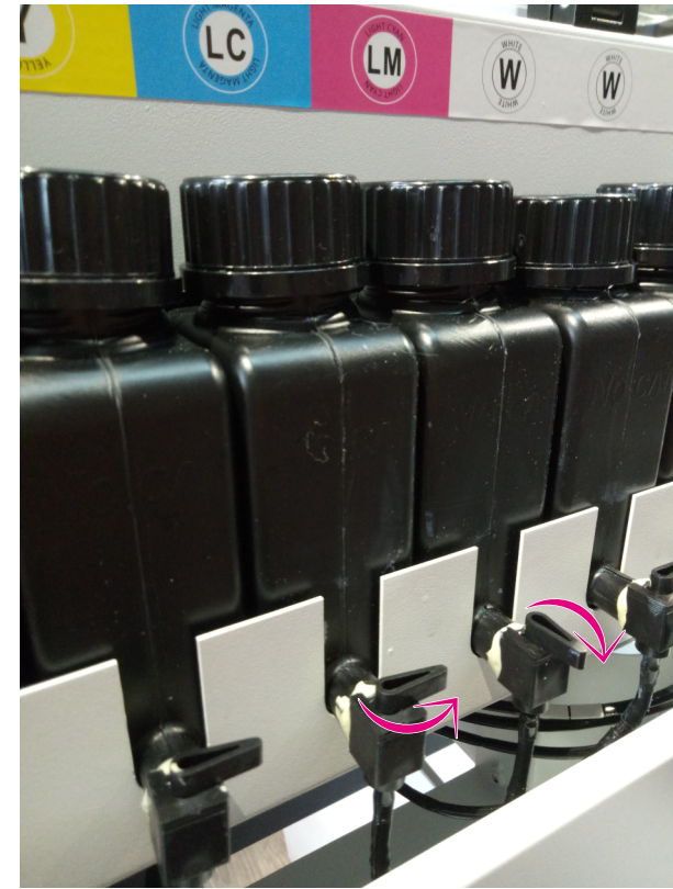
Turn to right Ink Supply. Turn to Left Stop Supplying.
